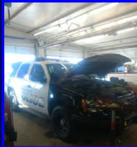
We replaced a tensioner pulley, an idler pulley and a belt. This rig is back in service.
