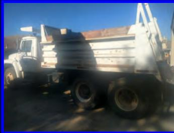
We installed the beaver tail so this truck is ready for chip seal.
