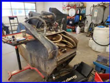
Work continues on the crusher bucket. We are pulling out the crushing plates and building them back up so that we can continue crushing cement this winter.
